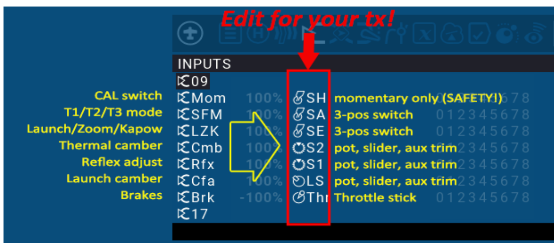
Figure 1 - screenshot of Inputs menu lines 10-16, showing control assignments
