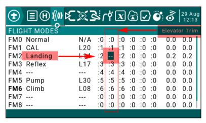
To test, enter Landing mode and move the elevator trim. There should be no system sounds.
